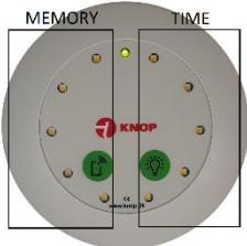
On the left side, there is a dim light where there is already a coded transmitter. The selected memory location is displayed with flashing. If an already encoded memory location is selected, it is overwritten.
