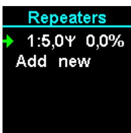
In this case, the added RP902 is shown on the top line as repeater "1". "1:5.0Y 9.9%", where 1=RP902 number, 5.0Y=antenna quality, 9.9%=rebroadcasts.
