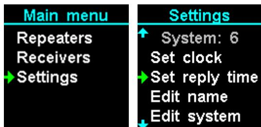
Select "**Reply time**" and press **Ent** to confirm. Press **Esc** to leave.
