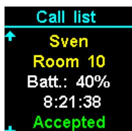
When an alarm is received from a transmitter that has, for example, a low battery, the message is displayed.
