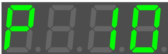
① Number of pulses/vibrations, e.g. 10, required to trigger an alarm.
