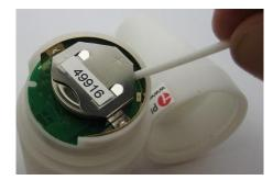
The battery is gently pushed out of the holder with the end of the for example a cotton swab or a match.
