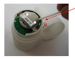
The battery is gently pressed out of the holder, for example with a cotton swab or a match. **Never use a metal object.**
