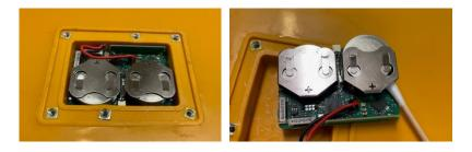
Then insert the printed circuit board and refit the cover.
